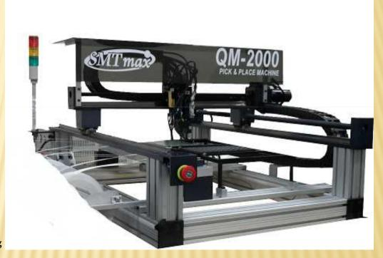
The QM2000 is a fully automated pick & place machine intended for SMT manufacturing and producing prototypes, developed by SMTmax. This remarkable, highly flexible and economical pick & place machine provides the need for a machine that produces small batches & prototypes for the SMT industry.
