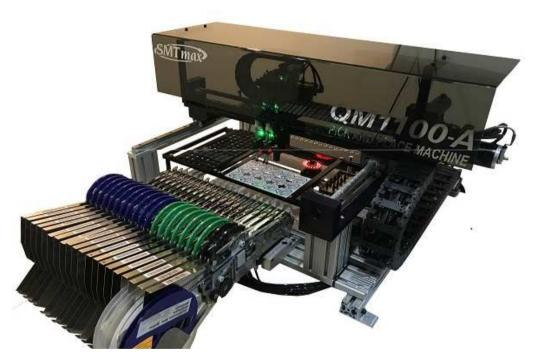
The QM1100-A is a fully automated pick & place machine intended for SMT manufacturing and producing prototypes, developed by SMTmax. This remarkable, highly flexible and economical pick & place machine provides the need for a machine that produces small batches & prototypes for the SMT industry.
